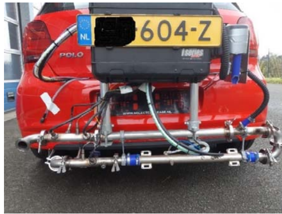
Figure 2-3: Flow measuring tube with dilution air pump and lambda, NO x -O 2 and NH 3 sensors.
